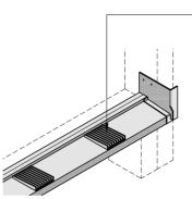
Apply PVC solvent cement to underside surface of the window support wedge & push firmly into place. Specific positioning requirements are dependant upon window frame & size refer Architects specification.
